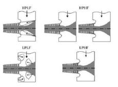
Picture-3: Typical nozzle locations and for online washing systems <sup>(15)</sup>.
