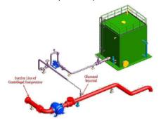
Picture-1: Compressor Chemical Cleaning
